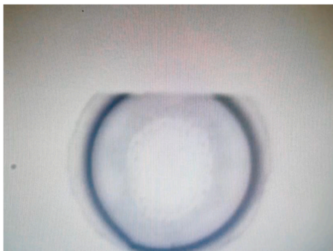
Fig. 2. Bright-field image of a partially ablated pL-droplet.
