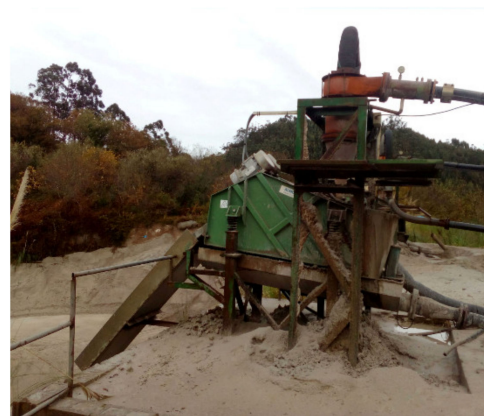
(b) Waste draining system
