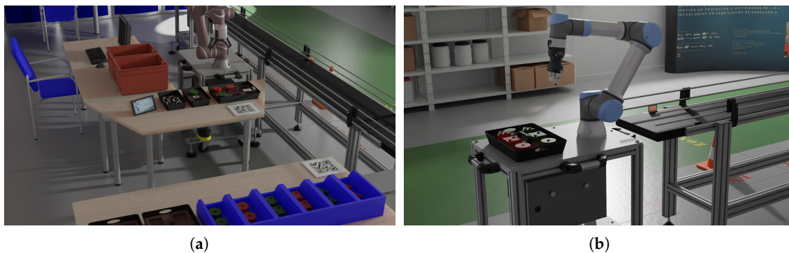
Figure 9. Virtual cell: (a) containers with the parts and assembly robot, and (b) delivery robot.
