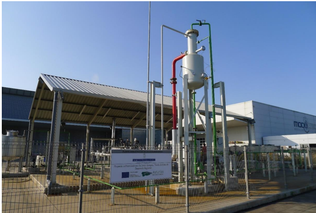
Figure 1. Hygroscopic cycle test plant with the steam absorber in first place.
