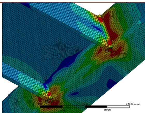
Fig. 5 FE model in ANSYS (Von Mises stresses)
