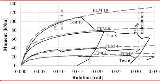
Fig. 8 Some  $M-\theta$  curves when fracture is observed
