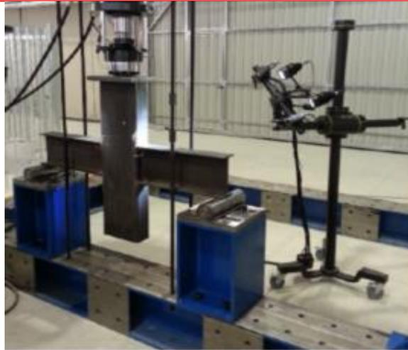
Fig. 3 Test rig with Aramis DIC system
