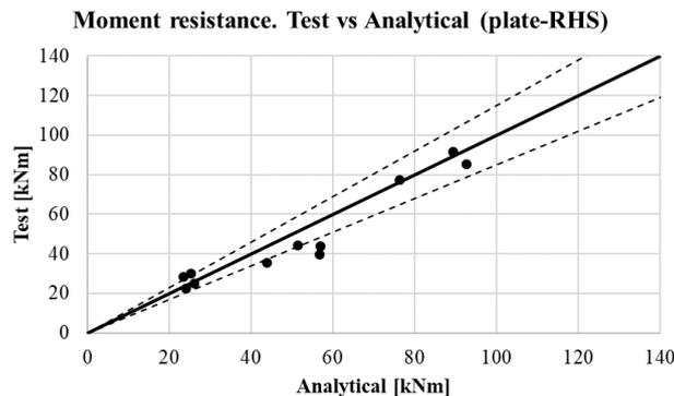
Fig. 18 Comparison of  $M_R$  from tests vs plate-RHS model
