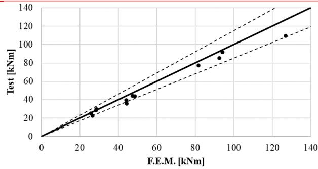
Fig. 7 Comparison of moment resistance  $M_R$  (tests vs FEM)
