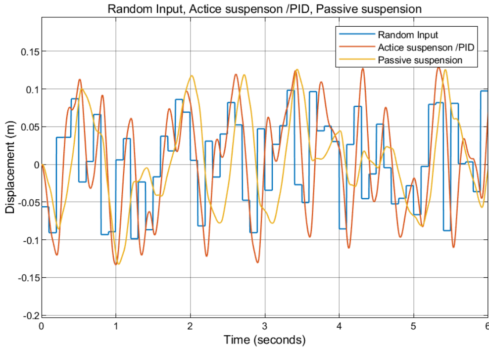
Figure 50. Passive vs PID Controller response for Random Input
