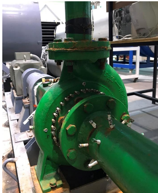
Fig. 2. Single volute commercial pump used for the present study.
