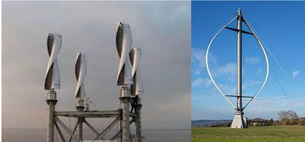
Figure 2.3. Savonius and Darrieus wind turbines
