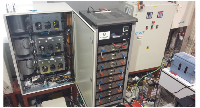
Fig. 4. Experimental setup. The figure shows the TAB and low-side converter as well as the ESS.
