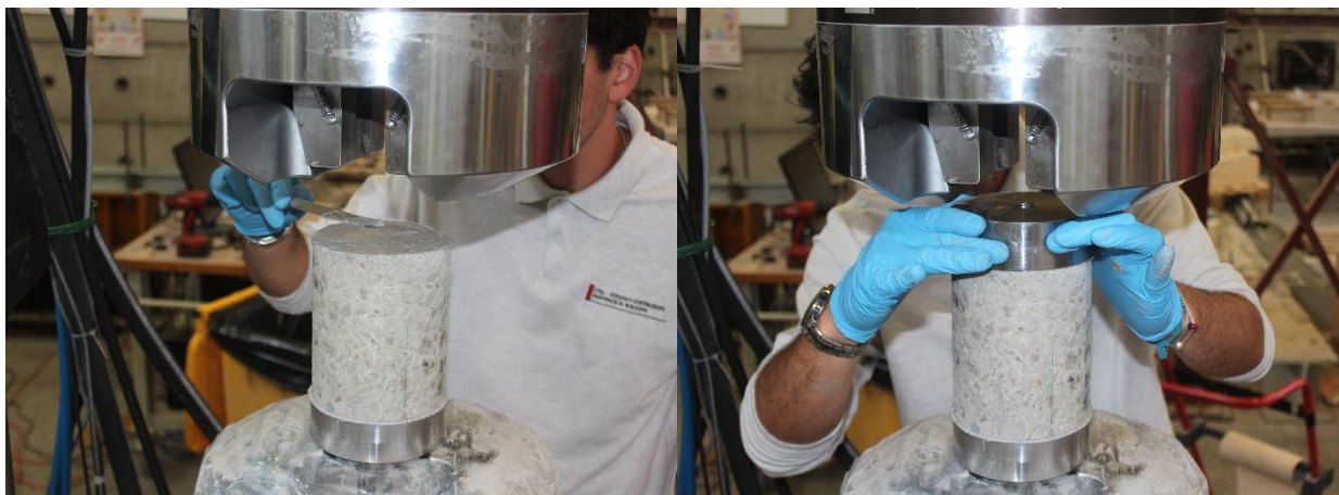
Figure 3.22- Gluing the top of the specimen
