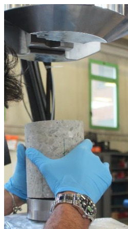
Figure 3.21- Placing the specimen in circular plate
