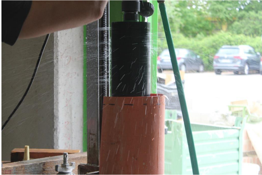
Figure 3.17-Removal of the cylinder in the machine
