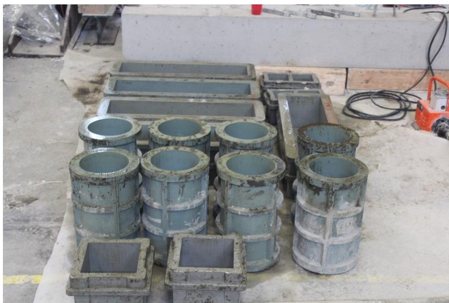
Figure 3.5-Formworks used concrete casting
