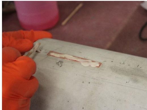
Figure 3.36- Gluing the strain gauges
