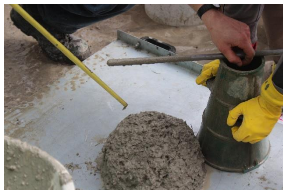
Figure 3.9- Test of lowering at the cone
