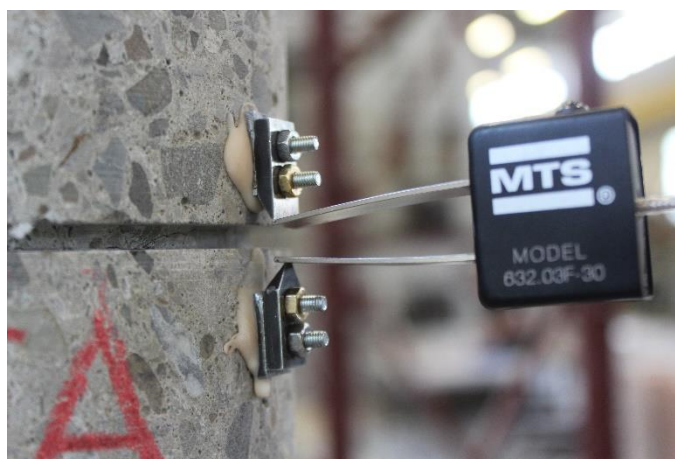
Figure 4.4-Clip-on gage transducer for measuring the crack opening.
