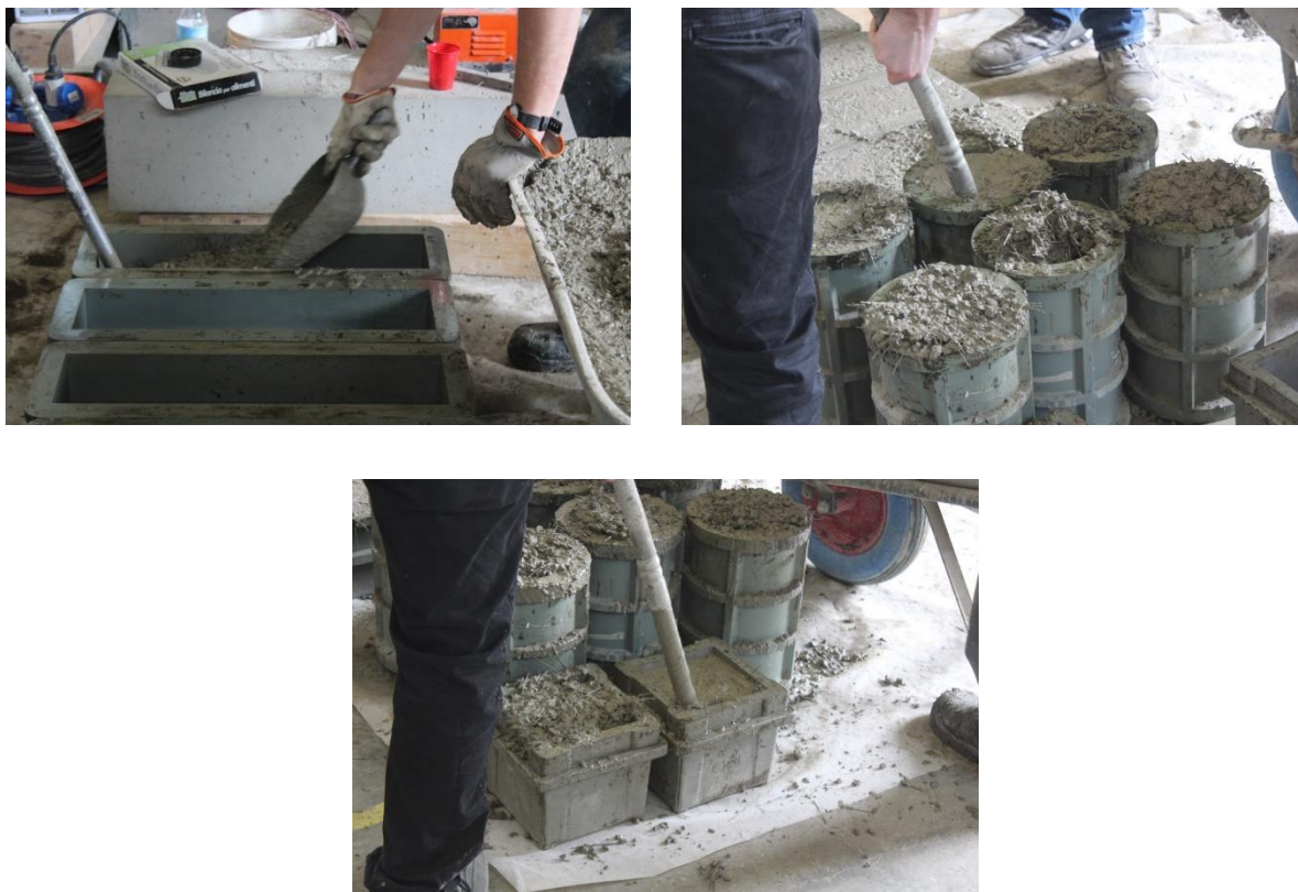
Figure 3.10- Vibration of concrete in the formwork
