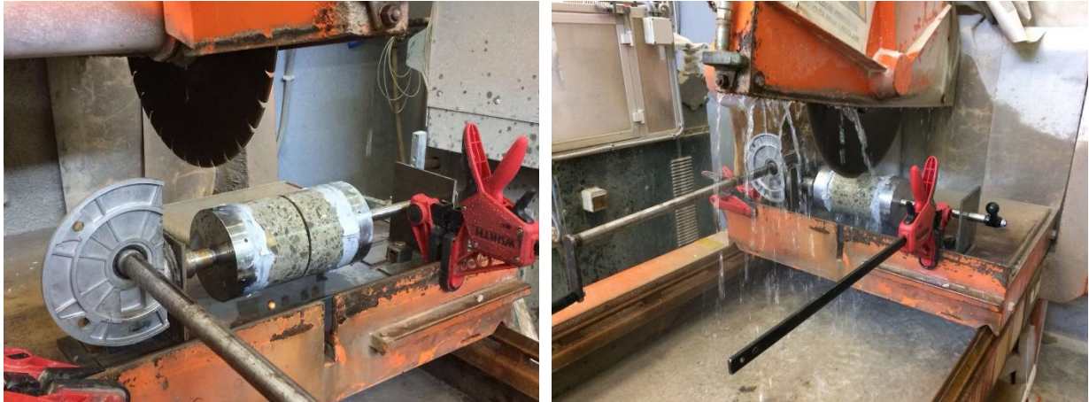
Figure 3.24-Disc saw and system for making notch
