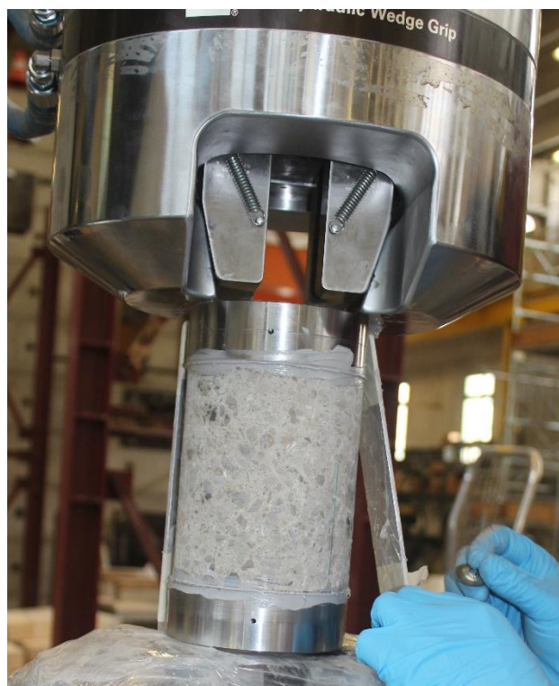
Figure 3.23-Union of the lower and upper part
