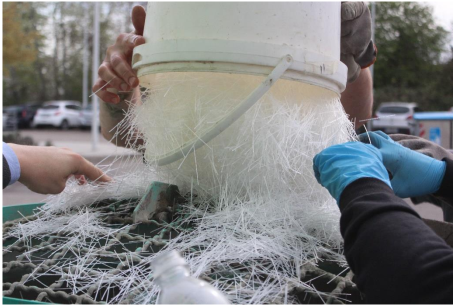
Figure 3.8-Addion of BASF fibres.
