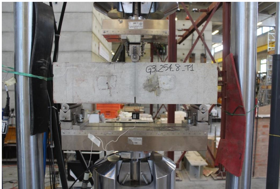
Figure 6.1-Three point test in beam specimen
