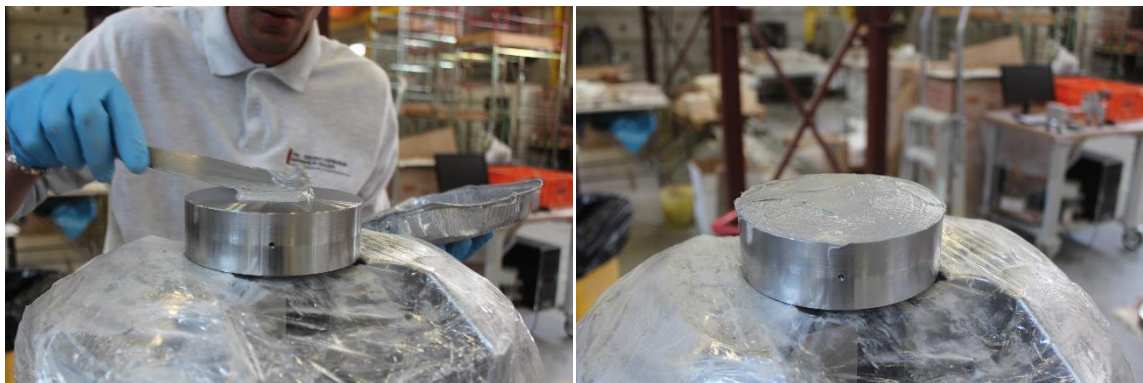
Figure 3.20-Gluing process of circular plate
