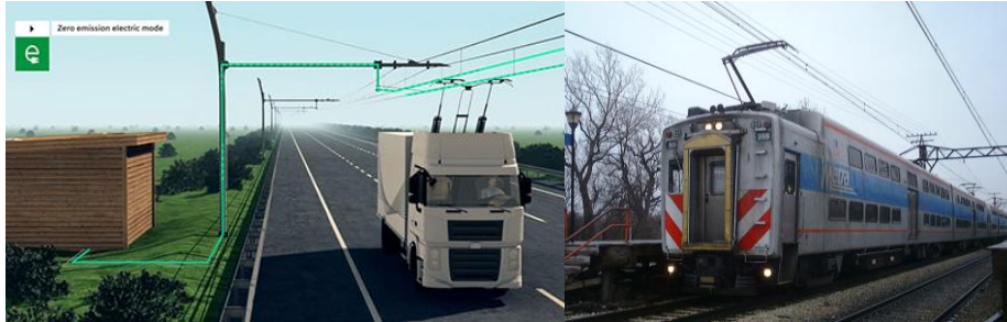
Figure 58 LHS Figure depicting operation of Siemens's eHighways scheme, where green indicates the energy flow path. RHS Figure depicting conventional electrified rail network architecture [242] [255].
