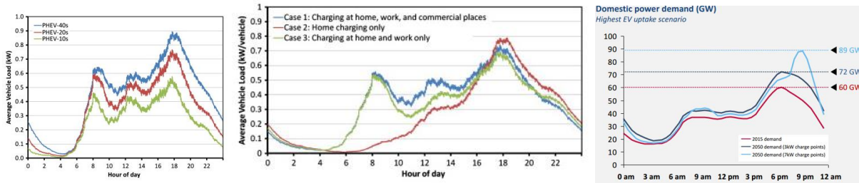
Figure 36 LHS Avg. vehicle load vs. capacity CENTRE Avg. vehicle load vs. charging strategy simulations [74]. RHS UK Government predictions for UK domestic power demand under max up-take scenario [88].
