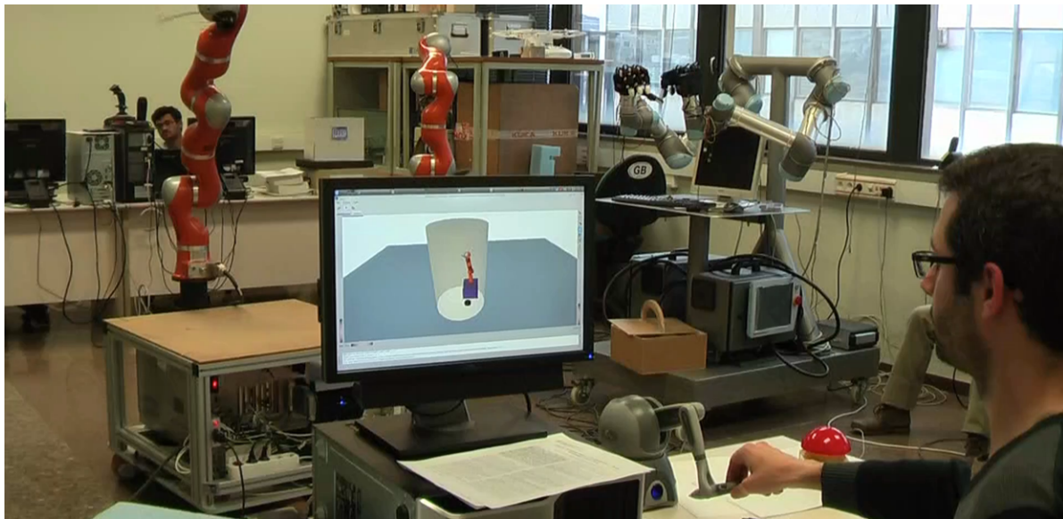
Figura 5: A scenario with a teleoperation task. The task is visualized in a virtual scenario.
