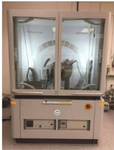
Figure 10. PANalytical Empyrean Diffractometer
