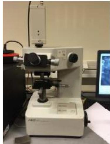
Figure 11. Hardness testing machine, Matzusawa
