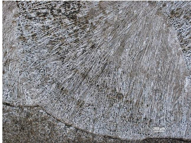
Figure 14. Castomag cladding after 20 seconds of etching. Magnification of 2.5
