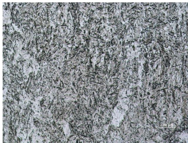
Figure 18. Corodur cladding after 10 seconds of etching with a magnification of 20
