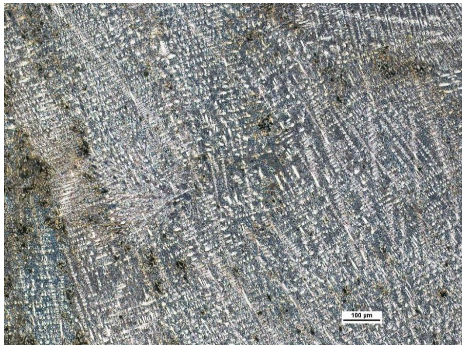
Figure 1. Hardface sample with a magnification of 10
