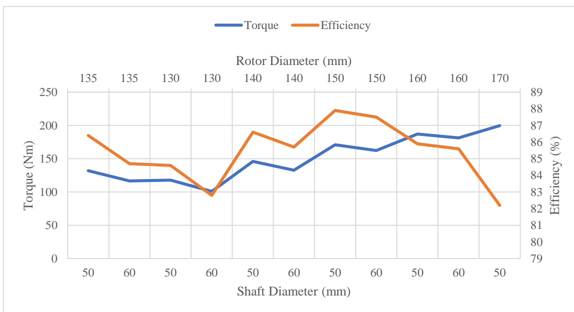
Fig. 3-5. Variation of rotor diameter and shaft diameter vs. Torque and Efficiency for D-1
