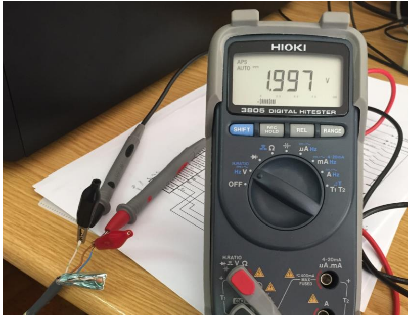
Figure 5.9 The multimeter measurement with 2V reference in the analog output test
