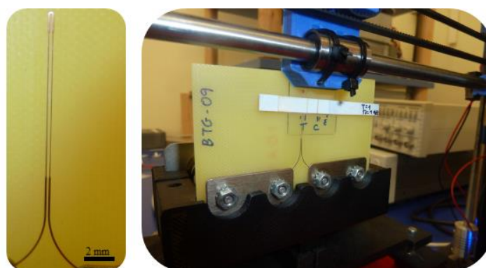
Fig. 2 Detail of the copper tracks (left) and photograph of the measuring system.
