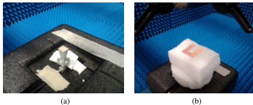
Figure 5. Measurement setup for the horn antenna with obstacle: a) antenna without any obstacle; b) antenna with a 'U' obstacle.
