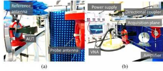
Fig. 13. Setup for the K a -band antenna measurement: (a) position of the antennas; (b) complete setup.
