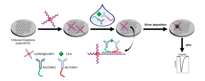
Fig. 4. Scheme of the immunosensor for CEA detection using a proximity ligation assay developed by Li et al. [74].
