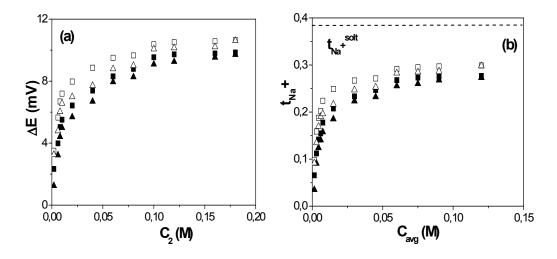
**Figure 3.** (a) Concentration potentials *versus*  $C_2$  solution concentration for the studied Al-Ox NPAM for both opposite external and solution stirring conditions; (b) Cation  $(t_+ = t_{Na+})$  transport number as a function of the average concentration  $C_{avg}$ . Dense symbols: stirred solutions; open symbols: non-stirred solutions. Solution cation transport number: dot-dashed line.
