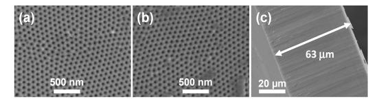
**Figure 1.** Scanning Electron Microscopy (SEM) micrographs of both membrane surfaces, (a) and (b), and cross-section (c) of the Al-Ox nanoporous alumina membrane (NPAM).
