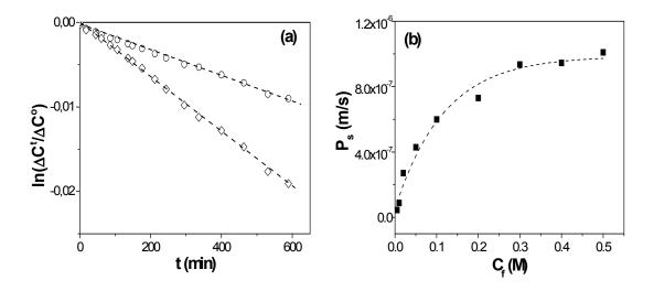
**Figure 2.** (a) Time evolution of solutions concentrations for  $C_f = 0.01$  M (o) and  $C_f = 0.1$  M ( $\diamond$ ); (b) Variation of diffusive permeability in the membrane with NaCl feed concentration.
