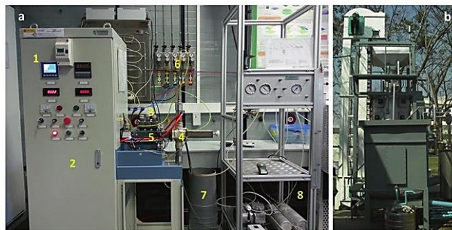
Fig. 6.3 a Microwave pyrolysis unit at lab-scale: 1 PID control panel; 2 cavity containing the magnetron; 3 tuning screws; 4 applicator-reactor; 5 waveguide; 6 thermocouple; 7 condensing system; 8 gas collecting system. b Continuous microwave biomass carbonization system. Reprinted with permission from [41], Copyright © 2014, Elsevier
