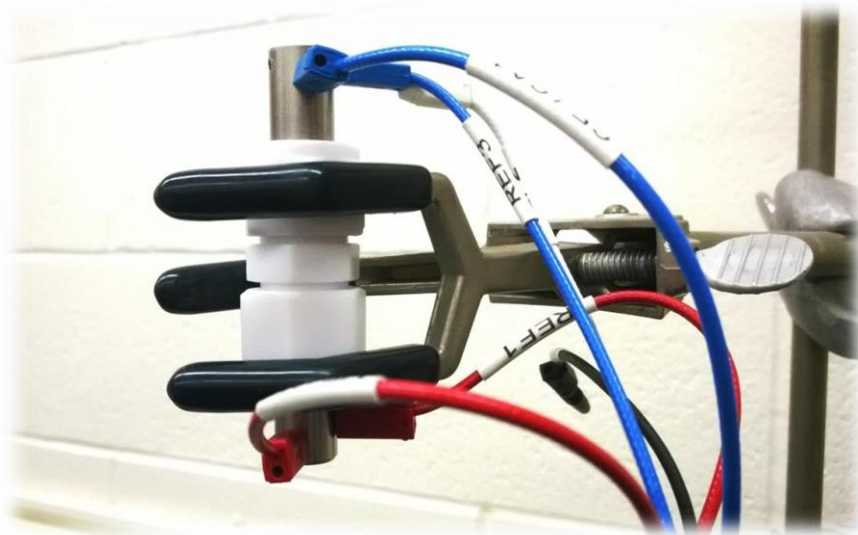
Fig. 5.9. Example of a Swagelok cell under test.
