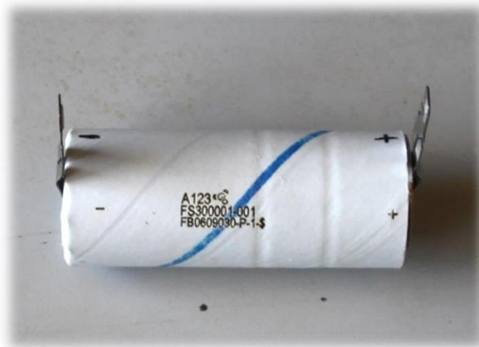
Fig. 5.1. Selected 2.3 Ah, high power GIC||LFP cell from manufacturer A123 Systems (model ANR26650M1).
