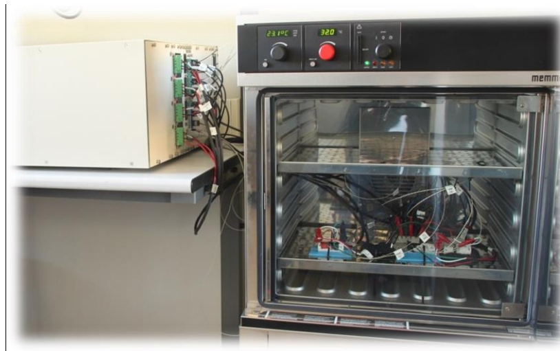
Fig. 5.11. Arbin BT-2000 testing machine (upper left) and the Memmert 1CP-500 climate chamber.
