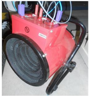
Figure 89: Fan Employed as the Resistive Load to be Fed by the DAB Converter.
