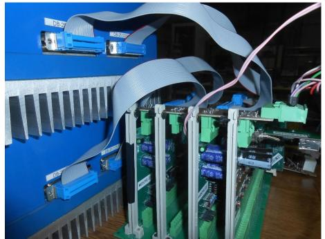
Figure 90: Backplane Structured Boards serve as the Programmer Hardware Interfacing the DAB Converter Power Stage with its Programmer Software.
