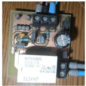
Figure 96: Relay Board.
