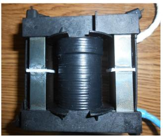
Figure 79: Designed High Frequency Inductor.
