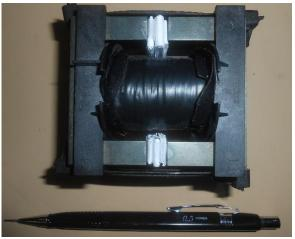
Figure 78: Designed High Frequency Inductor – Single Core.
