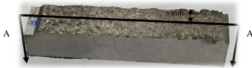
Figure 57. Fracture surface. Longitudinal section A-A.
