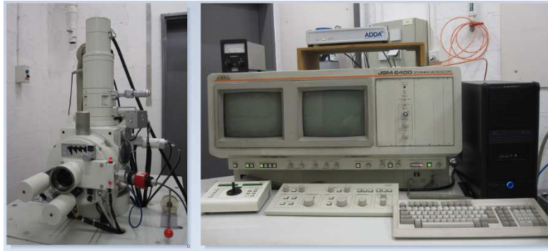
Figure 17. Scanning electron microscopy JSM-6400.
