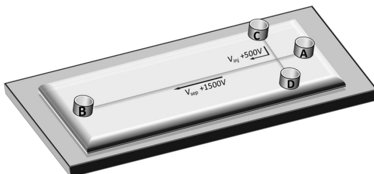
Figure 1. Scheme of the ME employed including the separation (A-B) and injection (C-D) voltage values.
