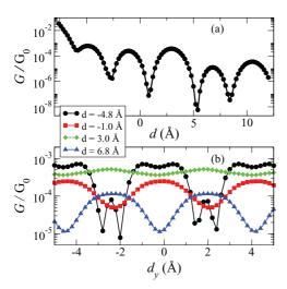
FIG. 4. (Color online) Low-voltage conductance  $G/G_0$  as a function of changes in the junction. (a)  $G/G_0$  as a function of the gap length d; (b)  $G/G_0$  as a function of the transverse coordinate  $d_y$ .  $G/G_0$  is estimated as  $T(E_{\rm F})$ , using only the  $\Gamma$  point in the k summation.
