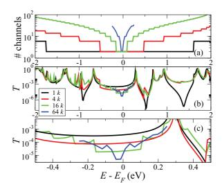
FIG. 5. (Color online) Convergence of the transport coefficients with the number of k points. (a) Number of channel as a function of energy; (b) T(E) for the d=3.0 Å junction; (c) Blowup of T(E) to show the convergency of  $T(E_F)$ . Black, red, and green lines correspond to 1, 4, and 16 k points, respectively.
