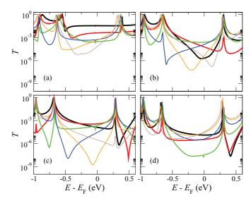
FIG. 3. (Color online) Evolution of the  $\Gamma$ -point transmission coefficient T(E) with increasing gap length d, which varies between -7.6 Å and +10.8 Å relative to  $d_0$ , in steps of 0.8 Å. Panels (a)–(d) correspond to curves in the intervals [-7.6 Å, -3.6 Å], [-2.8 Å, 1.2 Å], [2.0 Å, 6.0 Å], and [6.8 Å, 10.8 Å], respectively. Decreasing width of the lines corresponds to increasing d.
