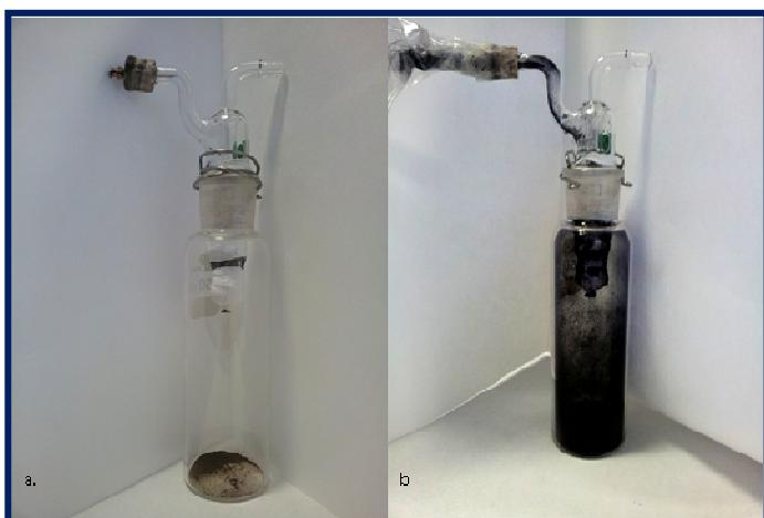
**Figure S1.** a) GO and b) TRG127 showing the explosion and the volume increase after blasting and the colour change from brown to black as a consequence of the thermal reduction.
