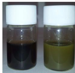
**Figure 2.** Images of GO-H (left) and GO-B (right) in water (without ultrasonication).
