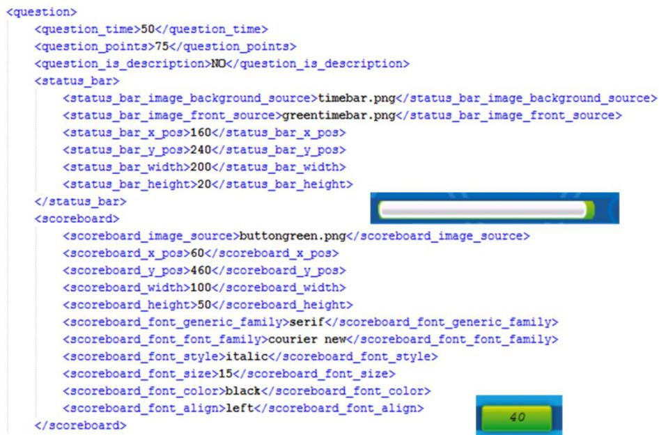
Figure 10 *Example of DSL containing the tags that define a time meter and a scoreboard.*
