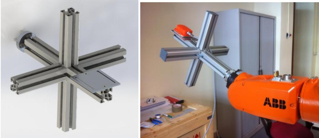
**Figure 2.** (Left) End effector designed to test several sensor units at once. (Right) Robot tool motion and sensor attachment.
