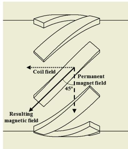
**Figure 7.** Resulting magnetic field on the strip.
