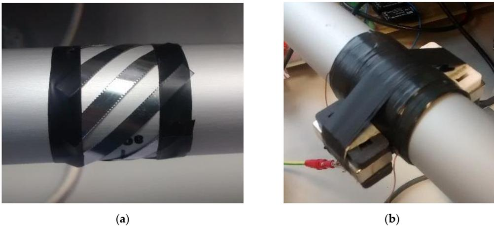
**Figure 8.** (a) Permendur strips attached around the pipe at 45°. (b) Transducer with coil and magnets.
