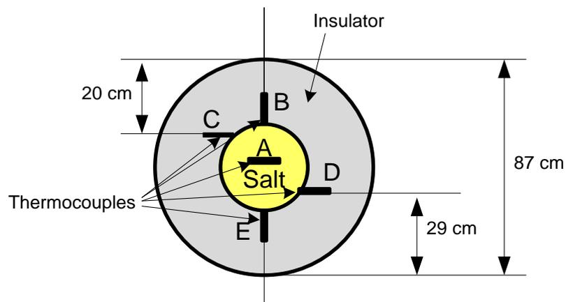
**Figure 2.** Cross section of the pipe and thermocouples position.
