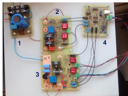
**Figure 13.** Experimental version of the power source. 1—Input rectifier. 2—Power bridge. 3—Auxiliar buck converter. 4—Control stage.
