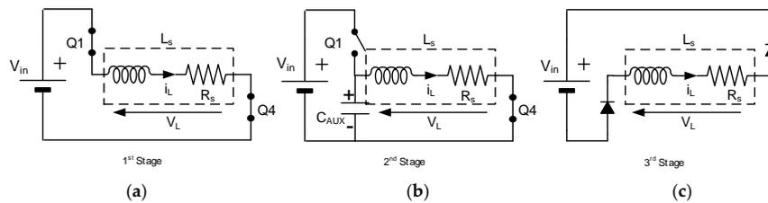
**Figure 11.** Full-bridge+buck converter stages: (a) First stage, (b) Second stage, (c) Third stage.
