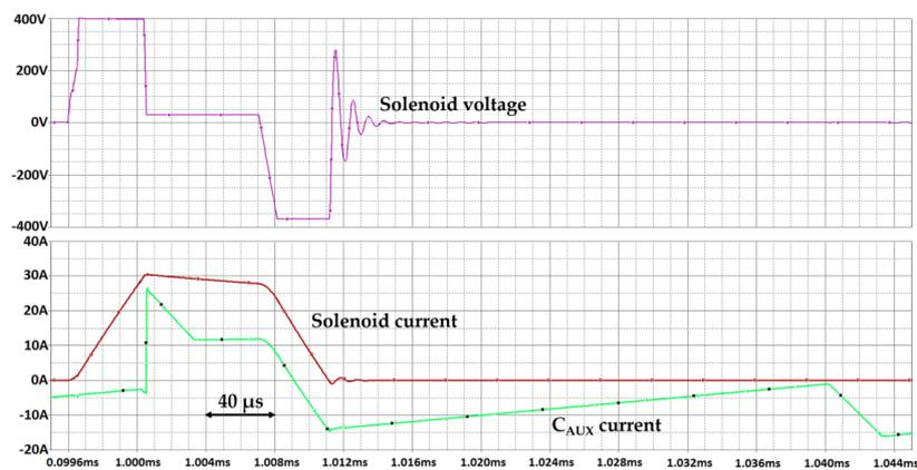
**Figure 12.** Simulated waveforms for the FB+buckpower supply.
