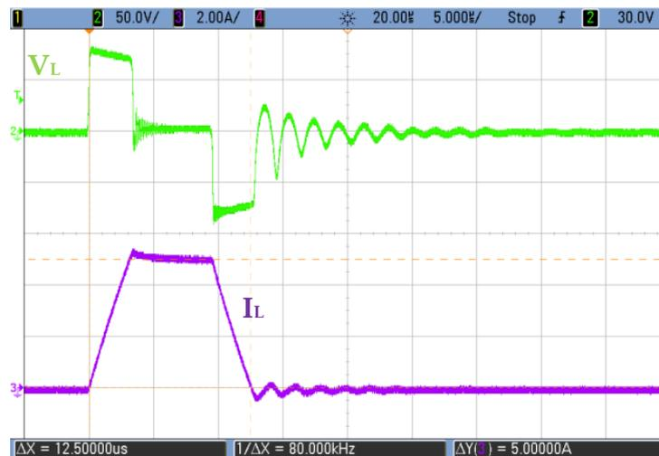
**Figure 16.** Trapezoidal current (Channel 3, purple) and voltage pulse (Channel 2, green) applied to the transducer by means of using full-bridge+buck converter.
