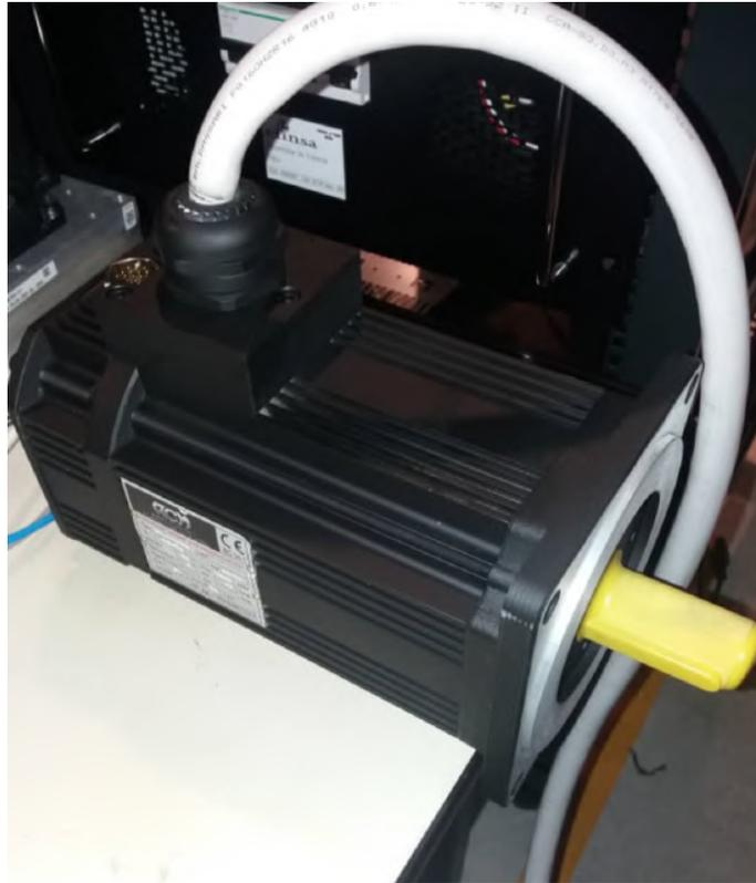
Figure B-4: ACM BRL110-3D 6 Poles Permanent Magnet Synchronous Electric Motor
