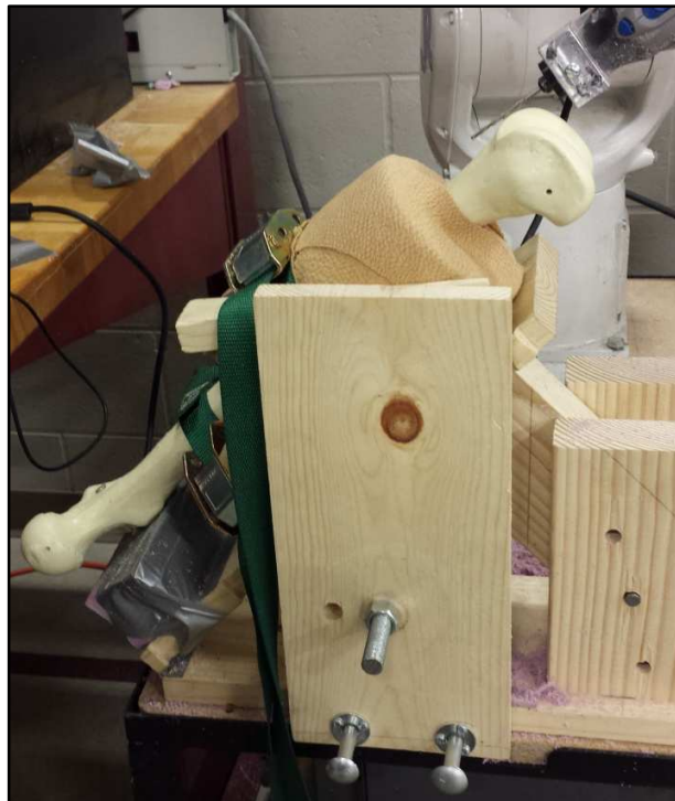
Figure 15. Testing station including final fixture, tool and leg model
