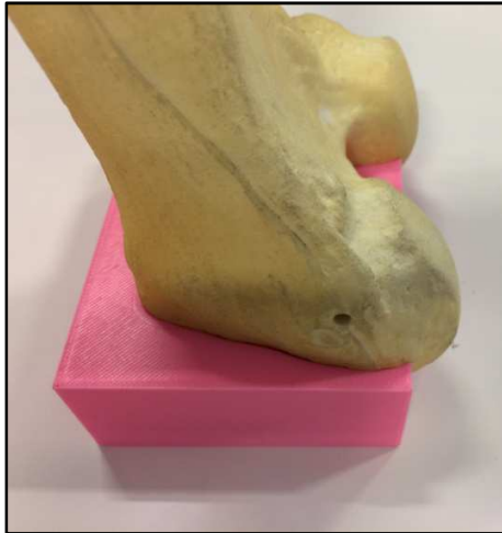
Figure 13. 3D printed mold fitting the sawbone
