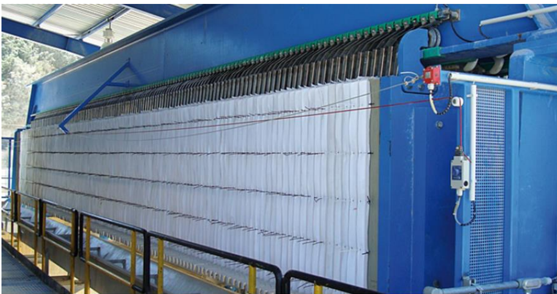
Figura 29: Filtro prensa (Advanced Mineral Processing S.L.)
