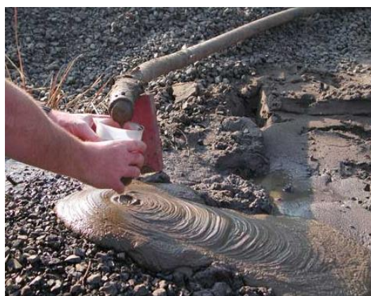
Figura 17: Relaves espesados (Paste Thick Associates, 2013)
