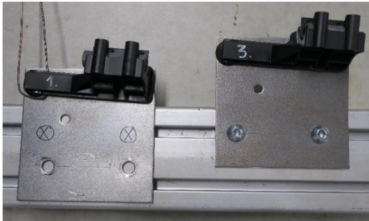
*Figure 40. Sample 1 with right hole's distance & sample 3 with wrong hole's distance.*
