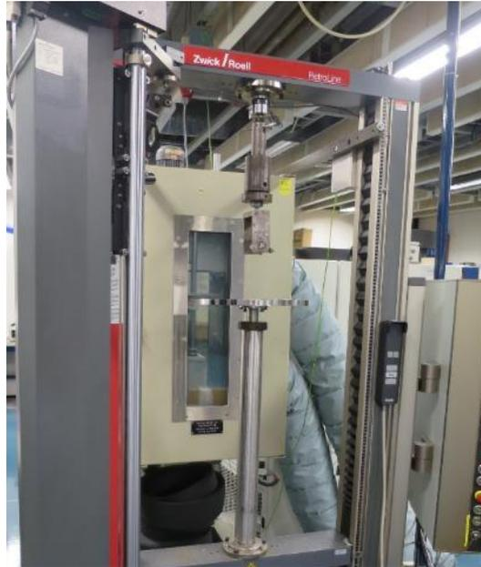
*Figure 41. Tensile machine and chamber at the back.*
