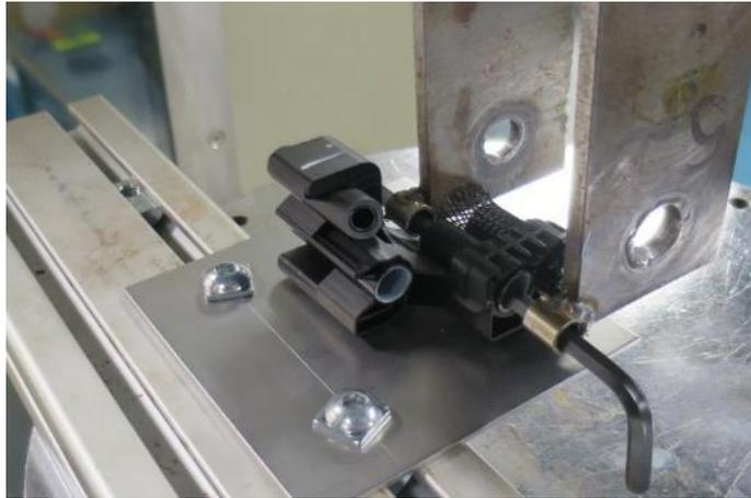
*Figure 42. Test of hole 3 with auxiliary tube in hole 4. New clip design.*
