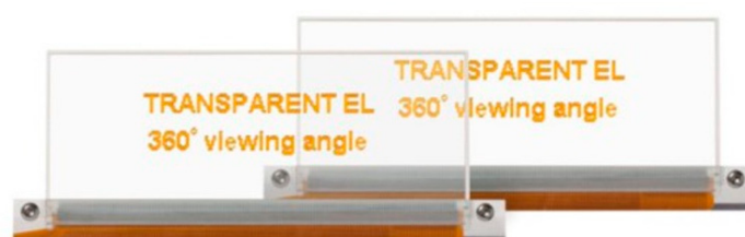
Figure 5. Fully transparent TFEL Display (by Beneq Oy, Finland).
