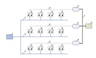
Figure 1: General structure of the distribution net of charging stations. It is formed by different parts such as: (1) power source, (2) three-phase electric power, (3) charging points, (4) masters, (5) server with database, (6) communication RS 485, (7) communication TCP/IP, (8) slaves.
