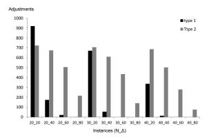
Figure 3: Number of adjustments of the maximum charge profiles depending on the type of the problems (type 1 or type 2), the maximum imbalance  $\Delta$  (0.2, 0.4, 0.6, 0.8) and the maximum number of active vehicles in one line N (20, 30, 40). The x-axis represents the group of instances for each type of problem ( $\Delta \times 100_{-}N$ ) and the y-axis the average number of profile adjustments made to solve the PI instances of each class.
