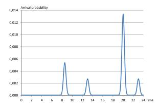
Figure 2: Arrival profile of vehicles along a day. x-axis represents the time of the day from 0 to 24 hours and the y-axis represents the arrival probability.
