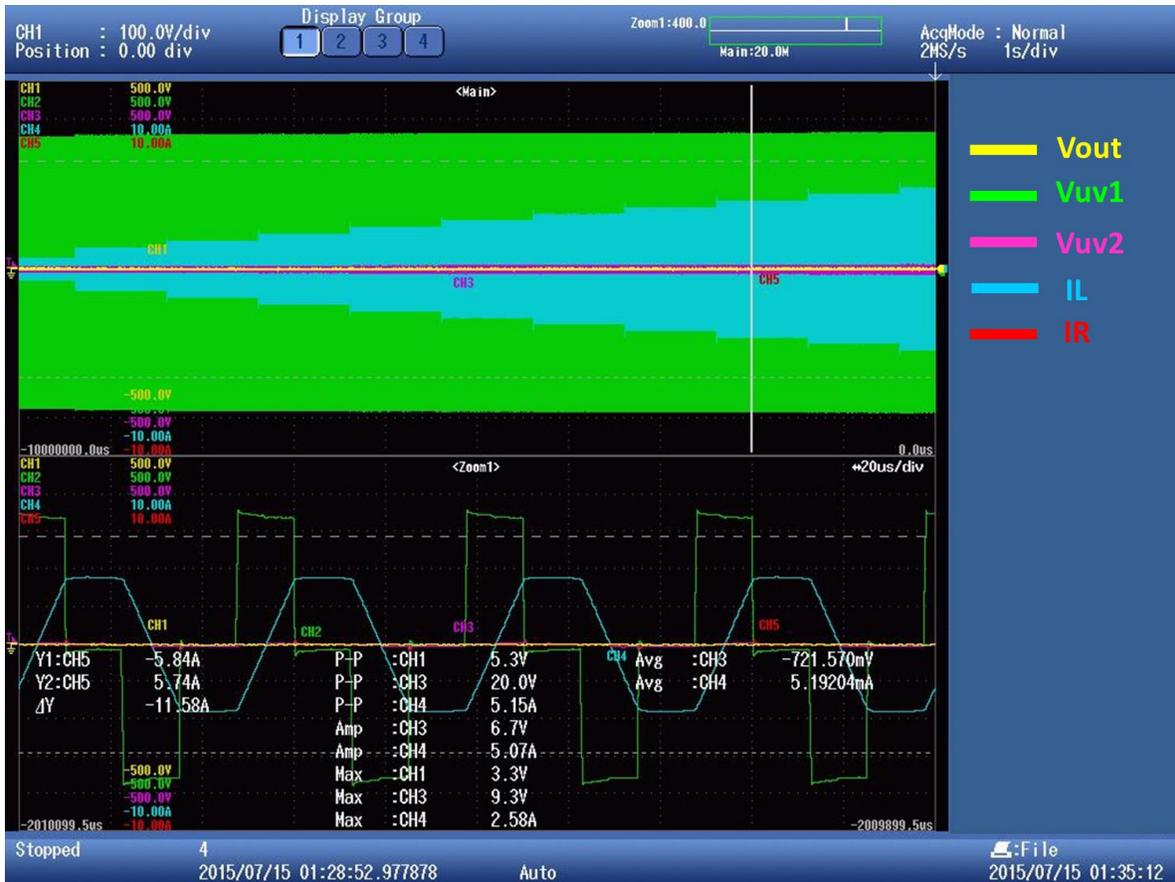
Figure 114: Soft Starting – Evolution of DPS Modulation Strategy a 9 degrees step increase Internal Phase until a Maximum of 180 degrees. The External Phase Shift is 0 degrees between Primary and Secondary Bridges.
