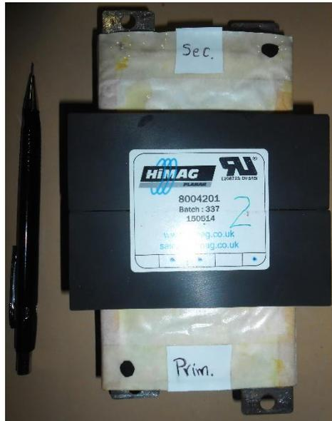
Figure 69: HIMAG High Frequency Planar Transformer.
