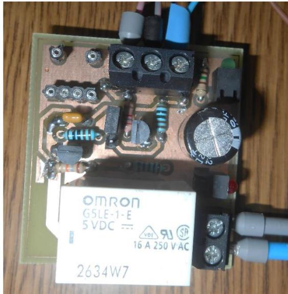
Figure 96: Relay Board.
