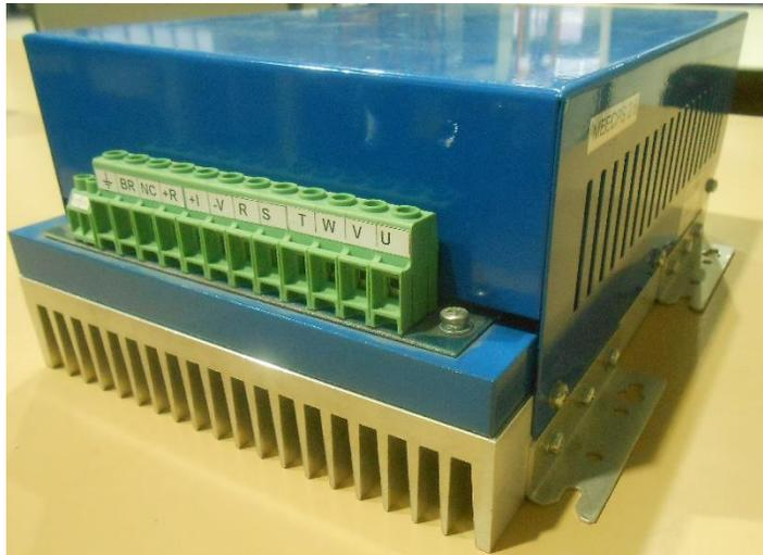
Figure 67: GUASCH MTL-CBI0010N12IXFE Converter-Brake-Inverter Power Stack.
