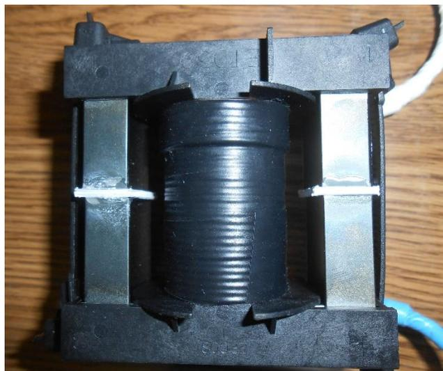
**Figure 79: Designed High Frequency Inductor.**
