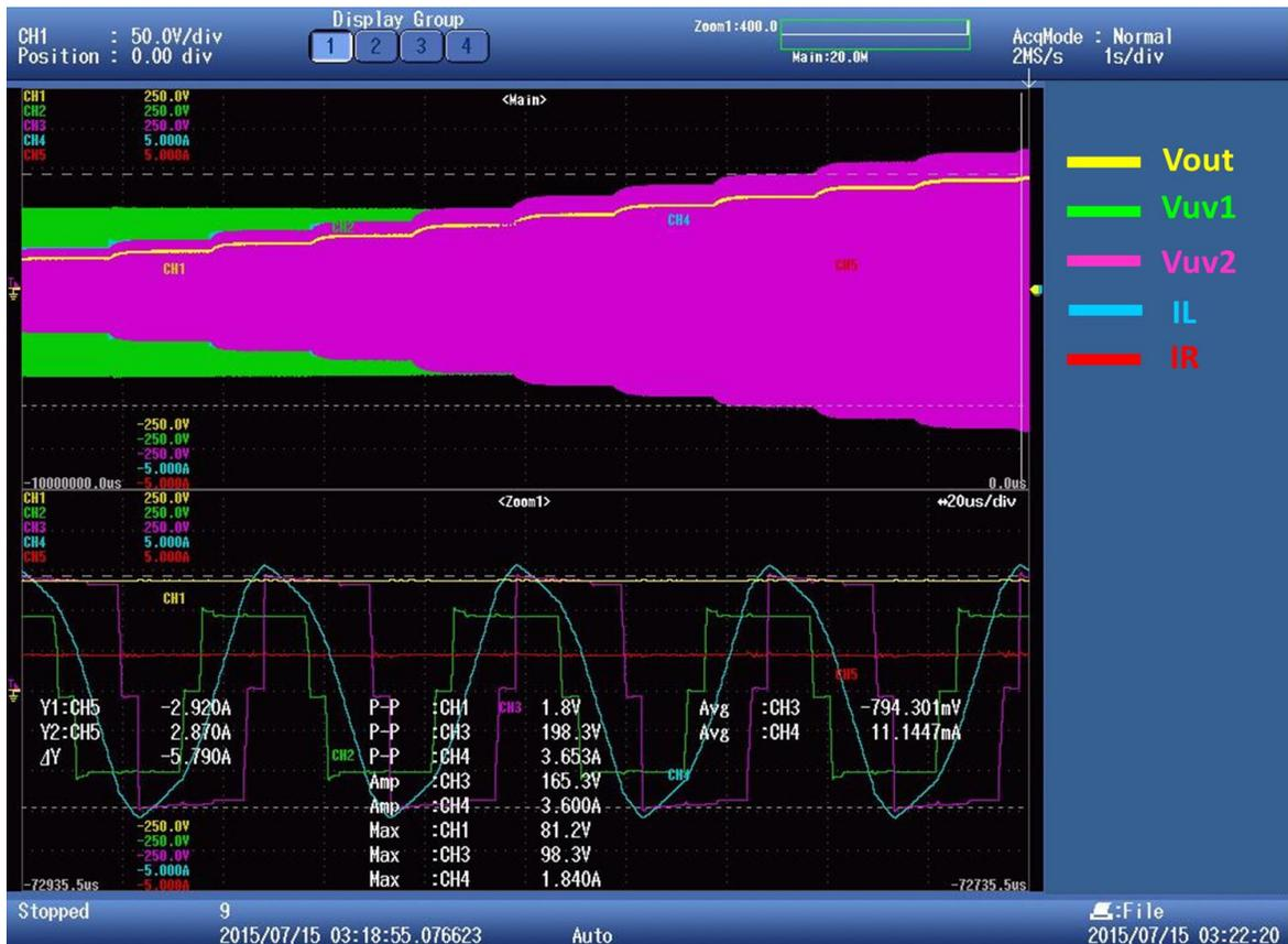
Figure 113: Soft Starting – Evolution of DPS Modulation Strategy a 9 degrees step increase Internal Phase until a Maximum of 180 degrees. The External Phase Shift is 90 degrees between Primary and Secondary Bridges.
