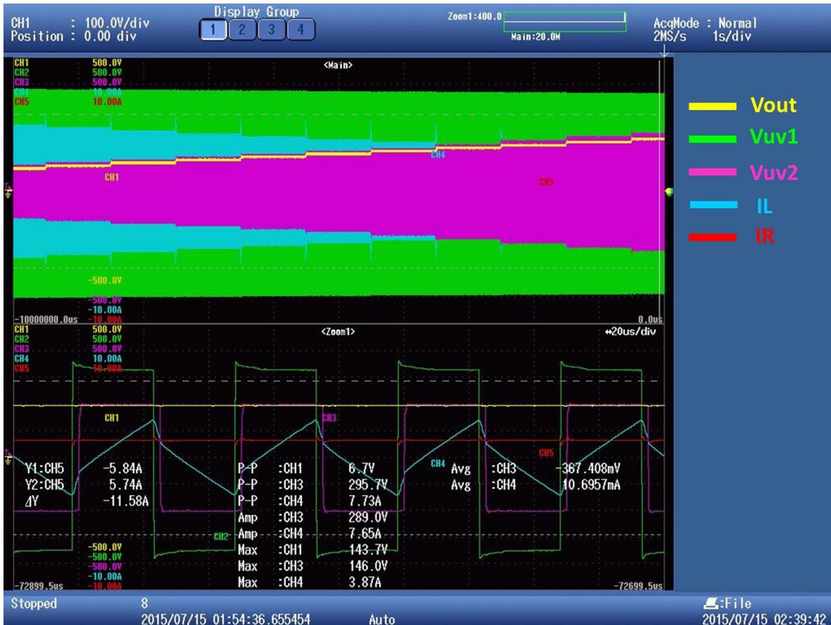
Figure 115: Gradual Increase of Voltage Reference Command, and Corresponding Reduction in Current Ripple as Output Voltage Increases in Response to the Reference.
