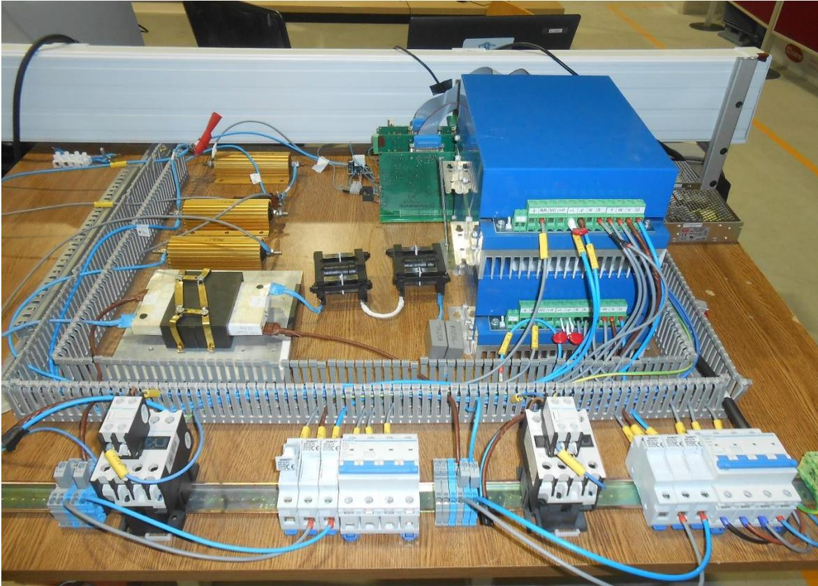
Figure 65: Constructed Experimental Platform for Practical Test of DAB Converter.
