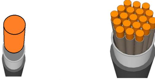
Figure 76: Inductor Design – Single versus Litz Wire.
