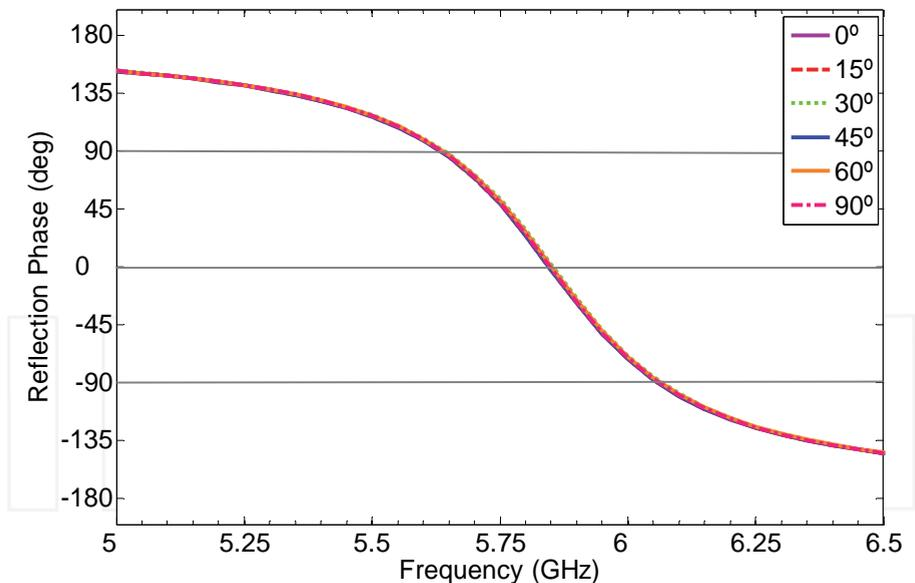
Fig. 2. Simulated Reflection phase of the AMC surface for different incident field ( $E_{inc}$ ) polarization angles  $\varphi=0^\circ, 15^\circ, 30^\circ, 45^\circ, 60^\circ$  and  $90^\circ$ .
