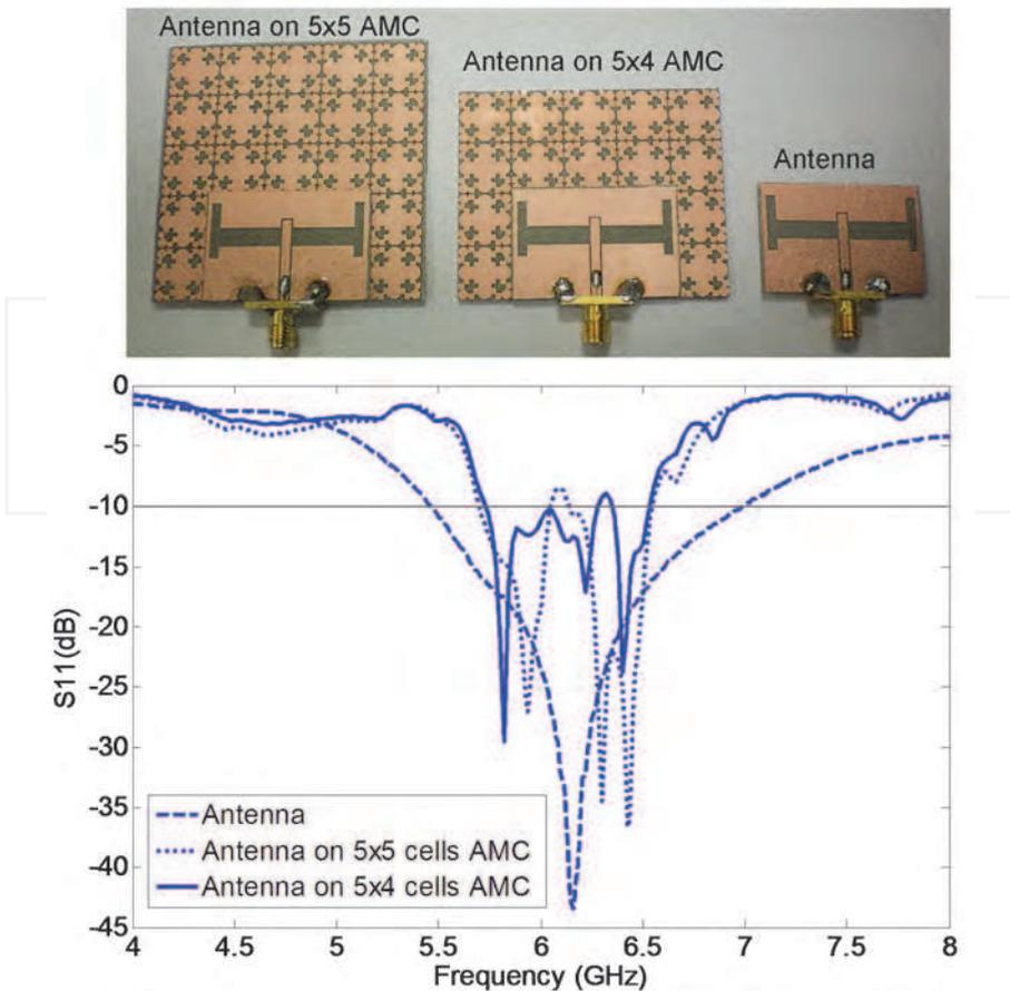
Fig. 6. Manufactured prototypes of the antenna on 5x5 cells AMC, the antenna on 5x4 cells AMC and the antenna (up). Return loss of the Antenna, the antenna on 5x5 cells AMC and the antenna on 5x4 cells (down).
