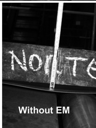
Fig. 8 - Example of strip edges with and without edge masking in similar strips (2mm thickness).
