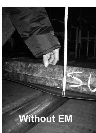
Fig. 8 - Example of strip edges with and without edge masking in similar strips (2mm thickness).
