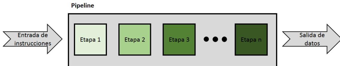
Figura 35: Estructura *Pipeline*
