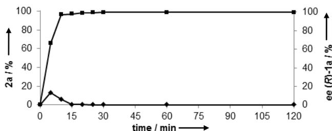
**Figure 2.** Time frame of the deracemisation of *rac*-1-phenylethanol (**1a**). Legend: **2a** (◆), ee(*R*)-**1a** (■).
