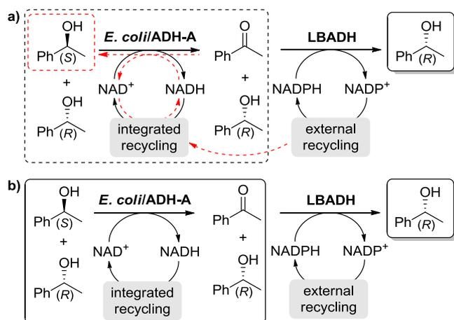
**Scheme 2.** Concurrent biooxidation and reduction processes for the deracemisation of *rac*-**1a** using: a) lyophilised *E. coli*/ADH-A cells; and b) resting *E. coli*/ADH-A cells; together with purified LBADH, external NADPH and a NADP cofactor recycling system. The undesired NADH-recycling catalysed by the external cofactor regeneration system in Scheme 2a is highlighted in red.
