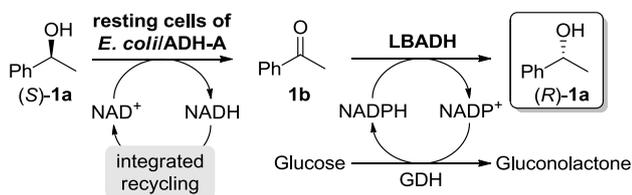
**Scheme 3.** Concurrent biooxidation and reduction processes for the stereoconversion of (*S*)-**1a**.
